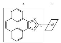
The A portion has a planar structure as a whole in that pyrene forms a fused ring, together with imidazole, pyrrole or pyrazine.
