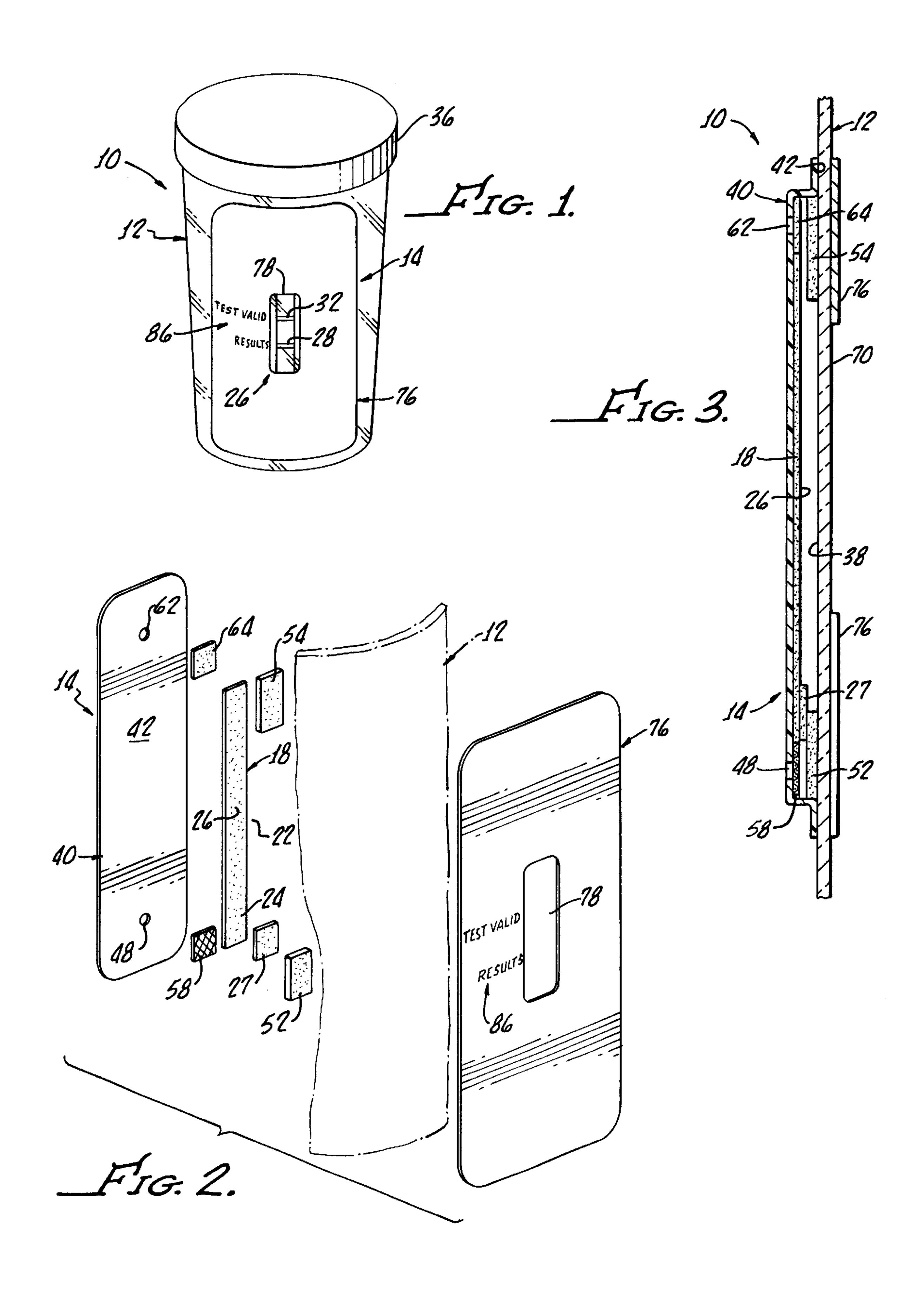
The present invention generally relates to diagnostic testing devices and more specifically relates to a device for containing a fluid sample, for example a urine specimen, and 5 conducting diagnostic testing of the contained fluid sample.
