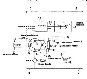
resistor connection of the load resistor. The semiconductor switch is connected by a second power connection to the second conductor and the link capacitor is connected by a second capacitor connection to the second conductor.
