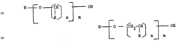
where the substituent R is hydrogen or lower alkyl containing from 1 to 5 carbon atoms including mixed substituents, and n is typically from 2 to 6 and m is from 10 to 100 or even higher. Included are poly-(oxytetramethylene) glycols, poly(oxyethylene) glycols, poly(oxy-1,2-propylene) glycols and the reaction 35 products of ethylene glycol with a mixture of 1,2-propylene oxide and ethylene oxide.
