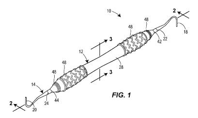
(57) Abstract: A dental instrument includes a handle and a tool that extends completely through the handle. The handle includes a handle body made of rigid material and a gripping sheath formed of resilient pliable material surrounding the handle body. The handle body and the gripping sheath may terminate at the same location on at least one end of the handle, preferably with an intersection with a bore through the handle body and/or an outer surface of a shaft of the tool.
