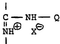
30 wherein Q is the residue from the amine used to react with the alkylated nylon and X is a counter anion. Where diamines are used, Q will be -R-NH<sub>2</sub> where R is preferably alkylene, phenylene, alkylphenylene, or phenalkylene.
