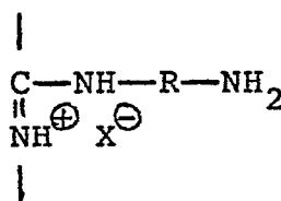
wherein R is alkylene, phenylene, alkylphenylene, or phenalkylene, and X is a counteranion.
