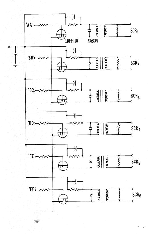
MULTIPLE PHASE RECTIFIER WITH ACTIVE FILTER FOR REMOVING NOISE IN TRIGGERING SIGNALS AND DIGITAL PHASE SHIFT COMPENSATOR FOR PHASE SHIFTING SIGNAL 5 PASSED THROUGH
