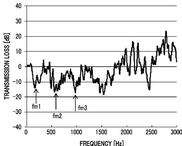
The soundproof system with a small size can obtain high transmission loss in a wide band.
