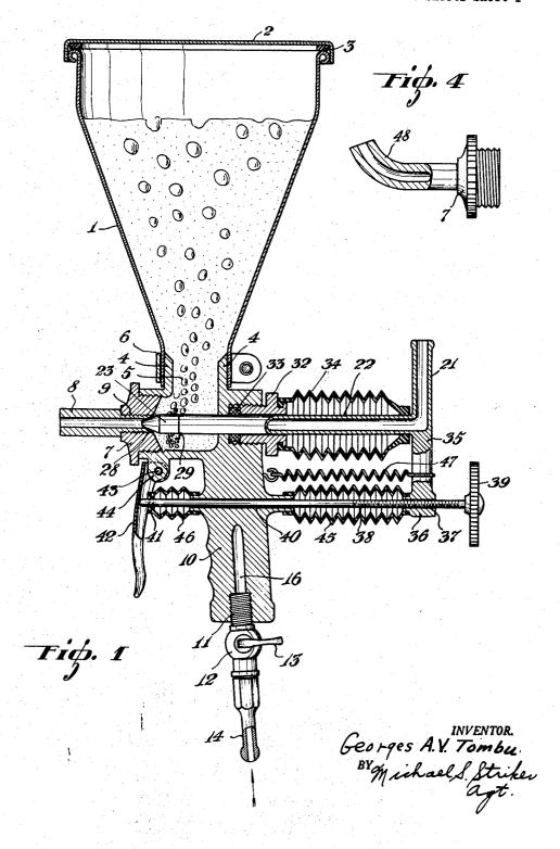
APPARATUS FOR PLASTERING WALLS BY MEANS OF COMPRESSED AIR
