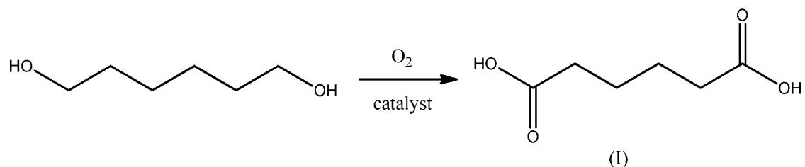
**[0025]** Catalysts suitable for the oxidation reaction (oxidation catalysts) are particular supported heterogeneous catalysts that include one or more metals on at least the external surfaces (the “exposed surfaces”) of a support, which metals are selected from platinum (Pt),
