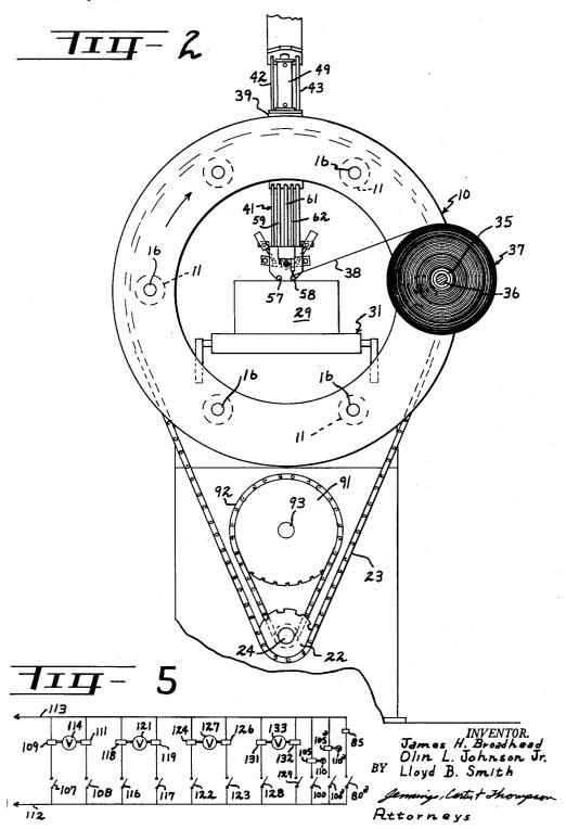
APPARATUS FOR WRAPPING ARTICLES WITH TAPE
