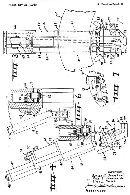
APPARATUS FOR WRAPPING ARTICLES WITH TAPE
