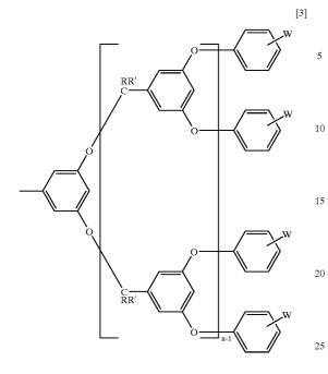
wherein R and R' each represent a hydrogen atom or a hydrocarbon group and may be identical or different, W represents an anionic group when the charge c is negative (–), or W represents a cationic group when the charge c is 30 positive (–), each W may be bound by a spacer molecule chain, and n represents an integer) and a water-soluble polyaminoacid-type polymer.
