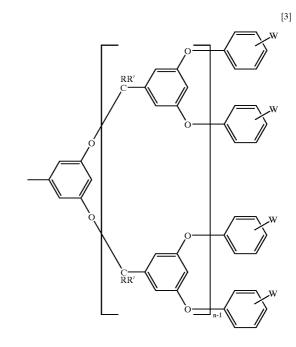
wherein R and R' each represent a hydrogen atom or a hydrocarbon group and maybe identical or different, W represents an anionic group when the charge c is negative (-), or W represents a cationic group when the charge c is positive (+), each W may be bound by a spacer molecule chain, and n represents an integer).
