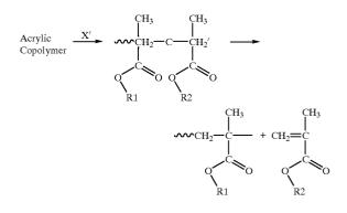
**[0025]** Since most acrylic resins for powder coatings are produced by free radical solution polymerization. The combination of high temperature, vacuum, and mechanical shear force during the devolatilization procedure deteriorates the resin products according to the mechanism of depolymerization shown above. The use of vacuum conditions, elevated temperature and high shear stirring to remove the solvent (and monomers) actually increases the rate of depolymerization.
