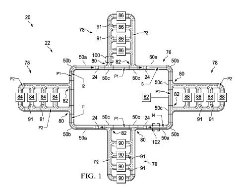
(57) Abstract: A system and method for simultaneously filling containers with different fluent products are disclosed. The system includes a plurality of vehicles that are independently routable along a track system to deliver containers to at least one unit operation station for dispensing fluent materials into the containers. The containers receive one or more fluent materials that differ from another in ingredients and/or weight percentage of at least one ingredient.
