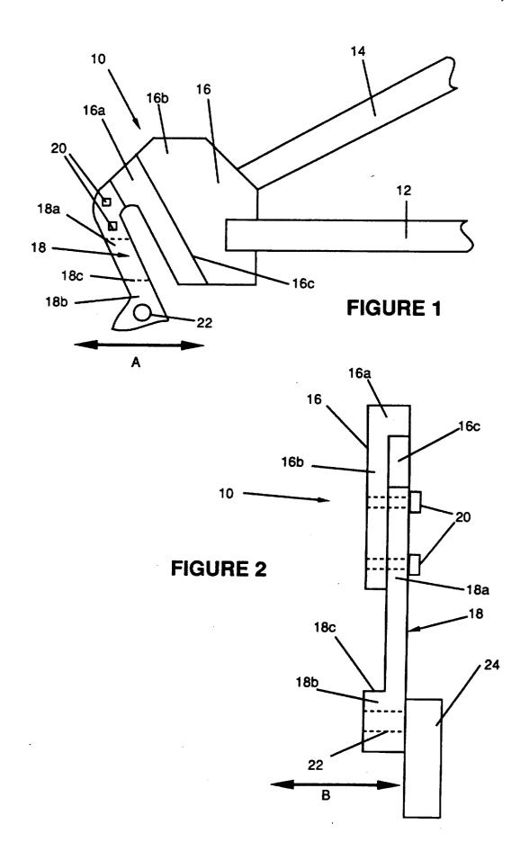
attached a derailleur plate 18 via an attachment means
