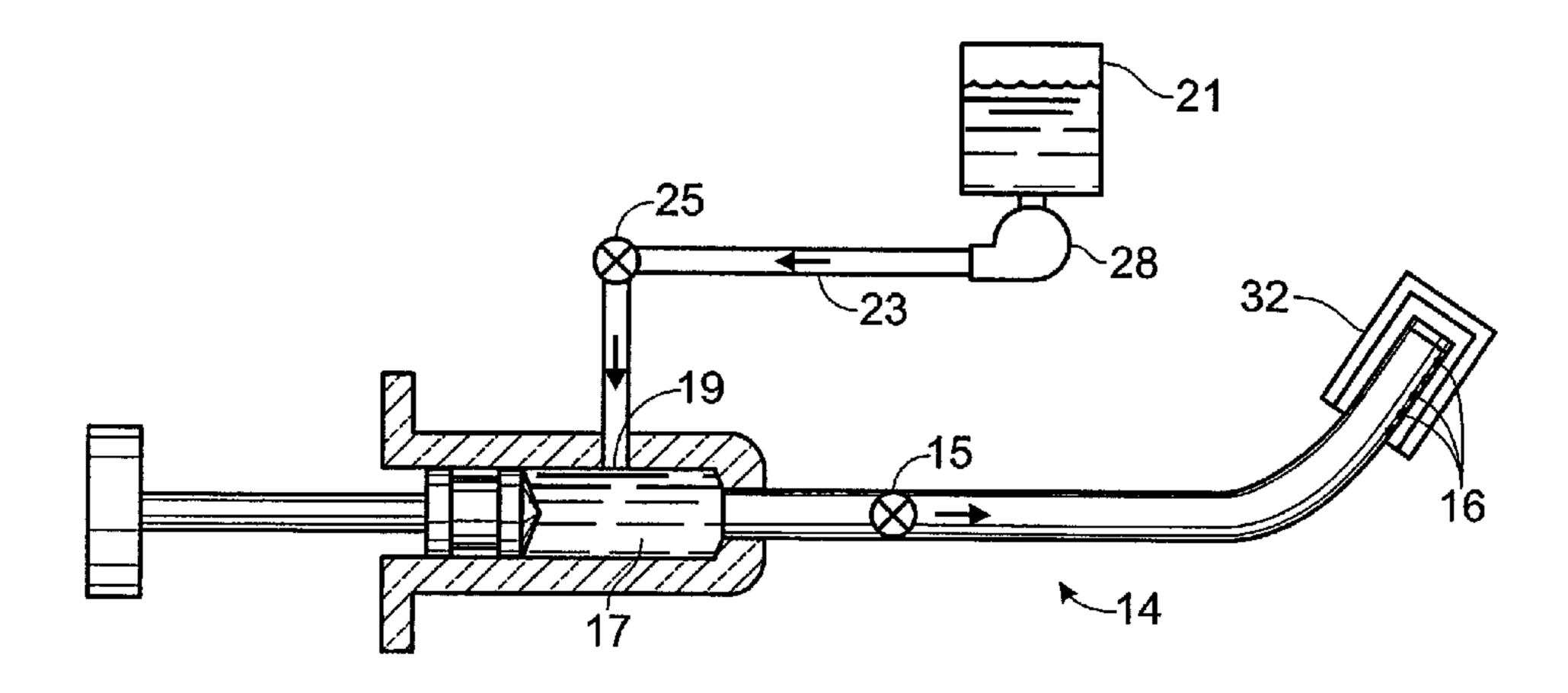
(57) Abstract: A needle-free injection system (10) is described. The needle-free injection system (10) may be suitable for injection into internal organs. In one embodiment, the needle-free injection system (10) includes an elongate end effector (14) that may or may not include a curved or angled distal end. The needle-free injection system (10) may include one or more orifices (116).
