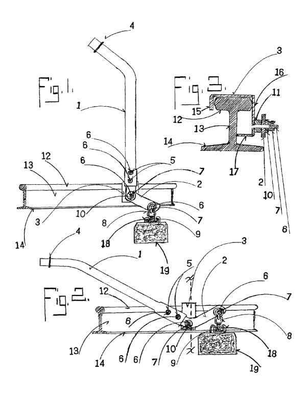
FIG. 2 Shows a side elevational view illustrating the tool in its active position
