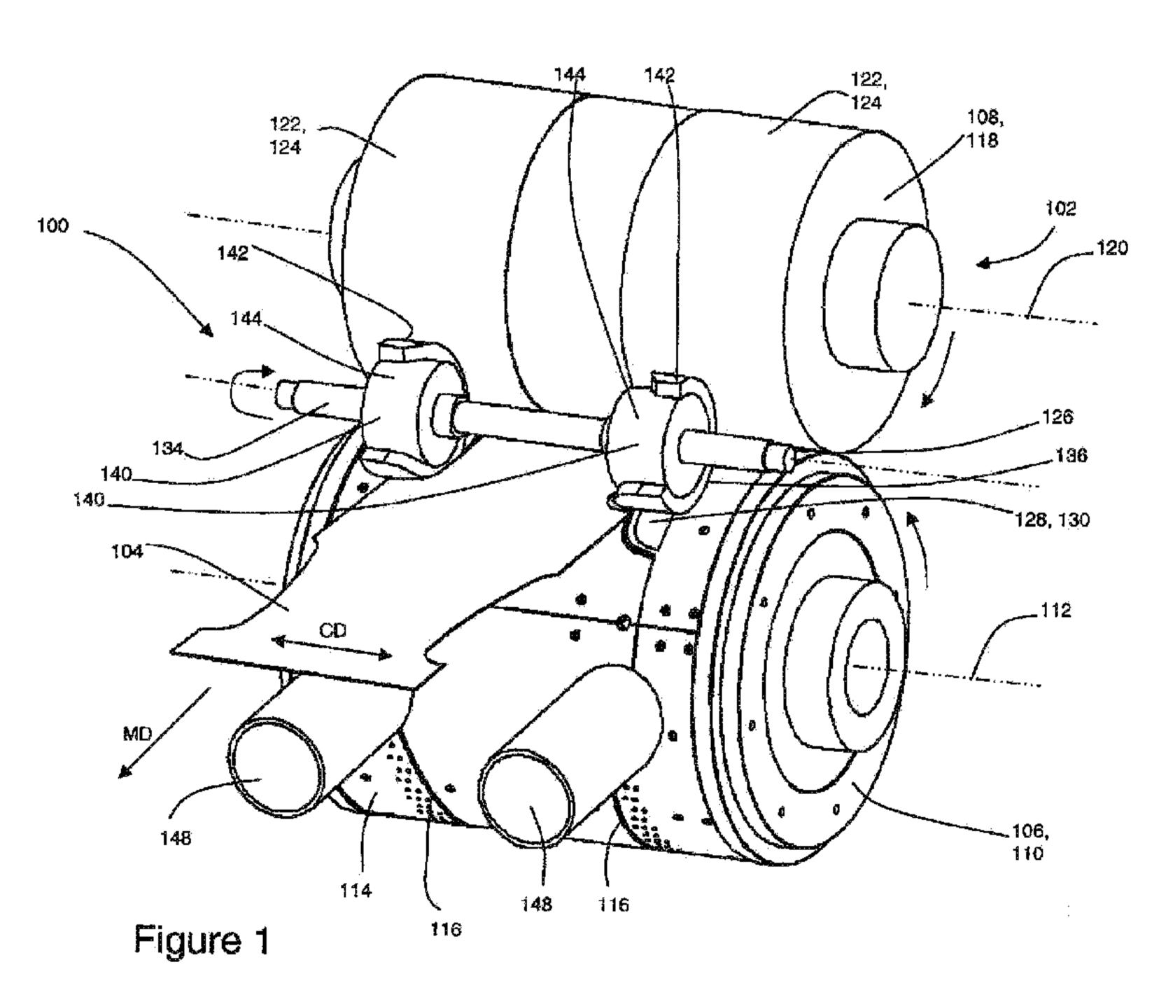
(57) Abstract: Aspects of the present disclosure involve methods and apparatuses for cutting and removing trim from an advancing substrate. Particular embodiments of the apparatuses and methods disclosed herein provide for removal of continuous lengths of trim, and in some embodiments, discrete pieces of trim from an advancing substrate.
