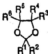
wherein each of R<sup>1</sup> to R<sup>6</sup> independently represents a hydrogen atom or a hydrocarbon group having 1 to 18 carbon atoms, and at least one of R<sup>1</sup> to R<sup>6</sup> has a structure of an ester or amide of (meth)acrylic acid as a substituent at a terminal thereof.
