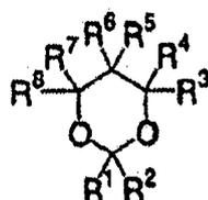
wherein each of R<sup>1</sup> to R<sup>8</sup> independently represents a hydrogen atom or a hydrocarbon group having 1 to 18 carbon atoms, and at least one of R<sup>1</sup> to R<sup>8</sup> has a structure of an ester or amide of (meth)acrylic acid as a substituent at a terminal thereof.
