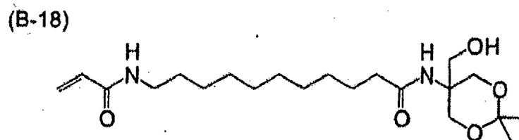
**[0017]** A content of the (B) specific polymerizable compound in the ink composition of an embodiment of the invention is in a range of 3 to 35 % by mass and, more preferably in a range of 4 to 25 % by mass on the basis of the total mass of the ink composition from the standpoints of a balance between a curing speed and an adhesion to the substrate and an inkjet adaptability of the ink composition.
