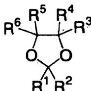
In Formulae (I) and (II), each of  $R^1$  to  $R^8$  independently represents a hydrogen atom or a hydrocarbon group. At least one of  $R^1$  to  $R^8$  in Formula (I) and at least one of  $R^1$  to  $R^6$  in Formula (II) respectively have a structure of an ester or amide of (meth)acrylic acid as a substituent at a terminal thereof.
