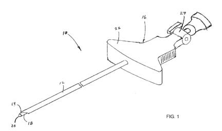
(57) Abstract: An endoscope (10) includes an outer tube (12) having a sharpened distal end (14) and a retractable sleeve (18) slidably disposed in the outer tube (12). An image conduit (20) is attached to the distal end of the retractable sleeve (18) for imaging any object in contact with the distal tip (26) of the image conduit (20).
