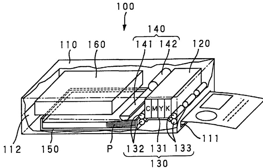
(57) Abstract: An inkjet printer (100) having a plurality of nozzles which discharge droplets of ink to cause them to land on paper (P), which landing results in dots recording information including characters and/or images. The inkjet printer (100) includes a line head
