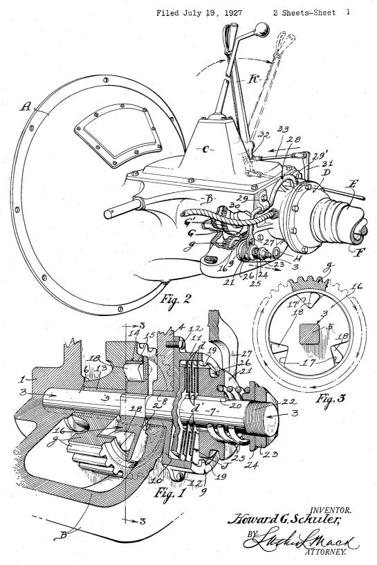
SAFETY CLUTCH MECHANISM FOR MOTOR VEHICLES
