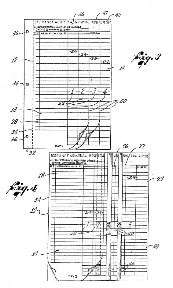
and attaching it to a retention sheet. The retention sheet includes a plurality of parallel adhesive strips by which the transfer sheets can be attached.
