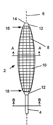
(57) Abstract: A surgical balloon is disclosed. The balloon can be woven, knitted or braided. The balloon can withstand extreme pressures relative to other surgical balloons. The balloon can have various geometries, including non-standard shapes. The balloon can be used to expand a support device. The balloon can be used to in an intrabone or interbone space to support bone. Methods of making and using the balloon are also disclosed.
