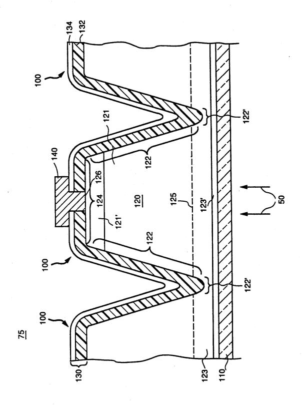
AVALANCHE PHOTODIODE WITH MOISTURE RESISTANT PASSIVATION COATING DISPOSED TO COVER THE OUTER PERIPHERY OF THE PHOTODIODE BODY EXCEPT AT A SELECTED TOP CONTACT AREA
