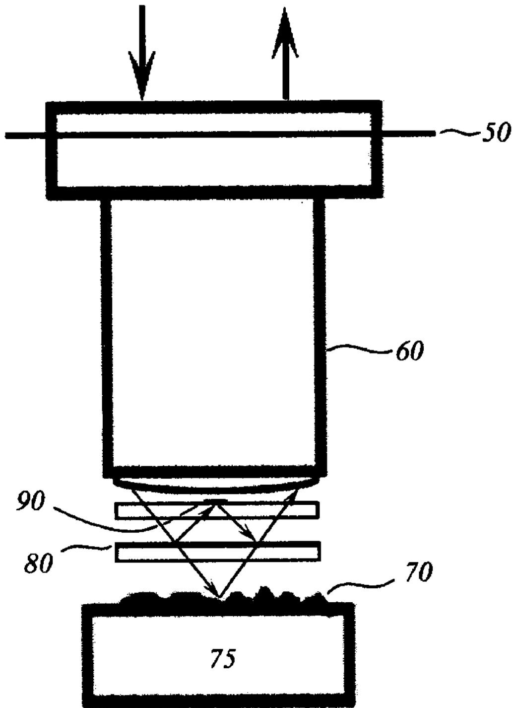
*specimen is mounted on a moveable stage capable of vertical motion in the diagram*
