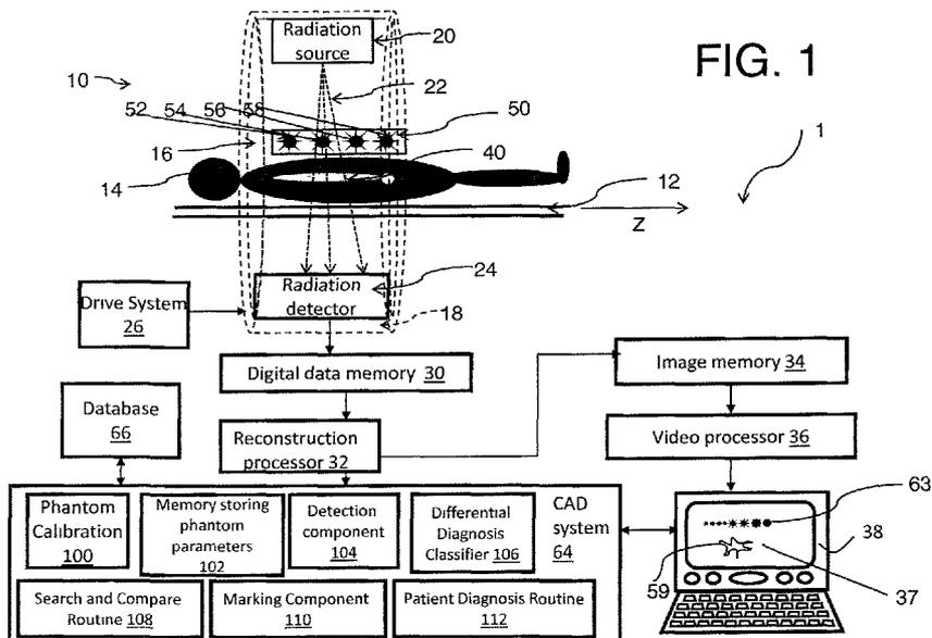
(57) Abstract: An imaging system (1) includes at least one hardware phantom (52, 54, 56, 58) which includes structural features (s, 82, 92) that mimic different structural features of tumors. A scanner (10) acquires image data for a subject (14) in a region of interest (40) and the at least one hardware phantom. A reconstruction processor (32) processes the image data to generate reconstructed image data representative of the region of interest and of the hardware phantom.
