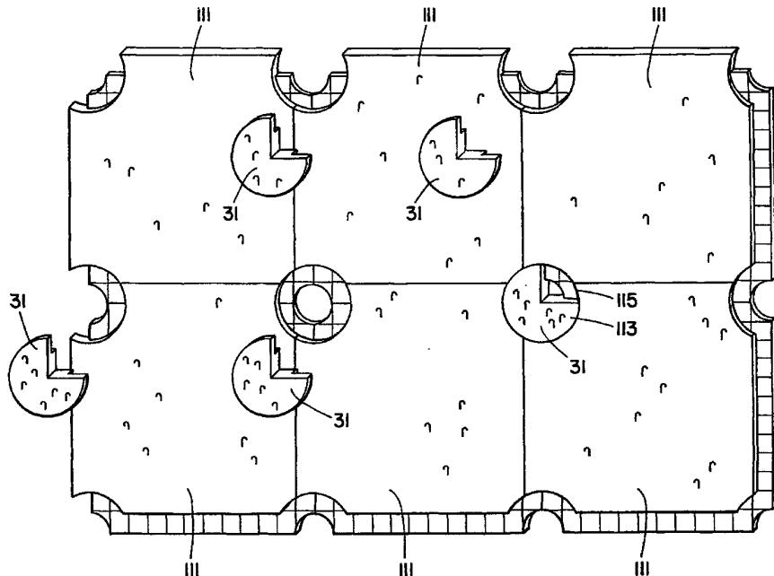
(57) Abstract: A method and apparatus for connecting anchor sheets to each other and/or to a floor is described. The approach involves using attachment pieces which fit into an area of reduced thickness of the anchor sheet which surround a cut away of the anchor sheet. In one embodiment, the attachment pieces are corner pieces which overlap areas of reduced thickness on a number of anchor sheets.
