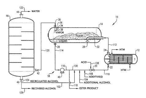
(57) Abstract: A polyester production process employing an esterification system that uses a distillation column to recover alcohol produced from an esterification zone and then recirculates the recovered alcohol back to the esterification zone without substantially cooling the recovered alcohol.
