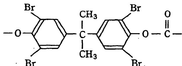
55 and the term "oligomer" as used herein means that having a polymerization degree (n) of 1 to 10. A flame retardant represented by the following formula:
