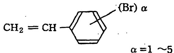
10 with 1 to 5 bromine atoms being bonded to the benzene ring of the styrene skeleton, and its polymer of the following formula:
