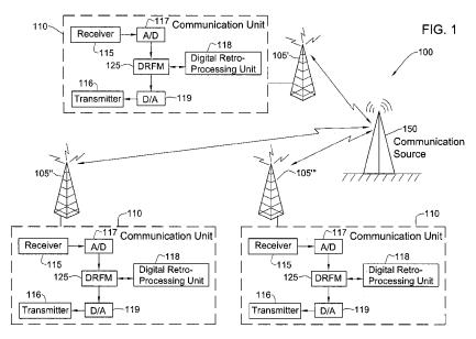
(57) Abstract: The present invention relates to a digital retro-directive system and method thereof for receiving incoming signals from a transmitting source by means of at least two antennas and transmitting outgoing signals back, substantially simultaneously, towards said transmitting source through said at least two antennas irrespective of the location of one antenna with respect to another and without calculating phase differences between said outgoing signals.
