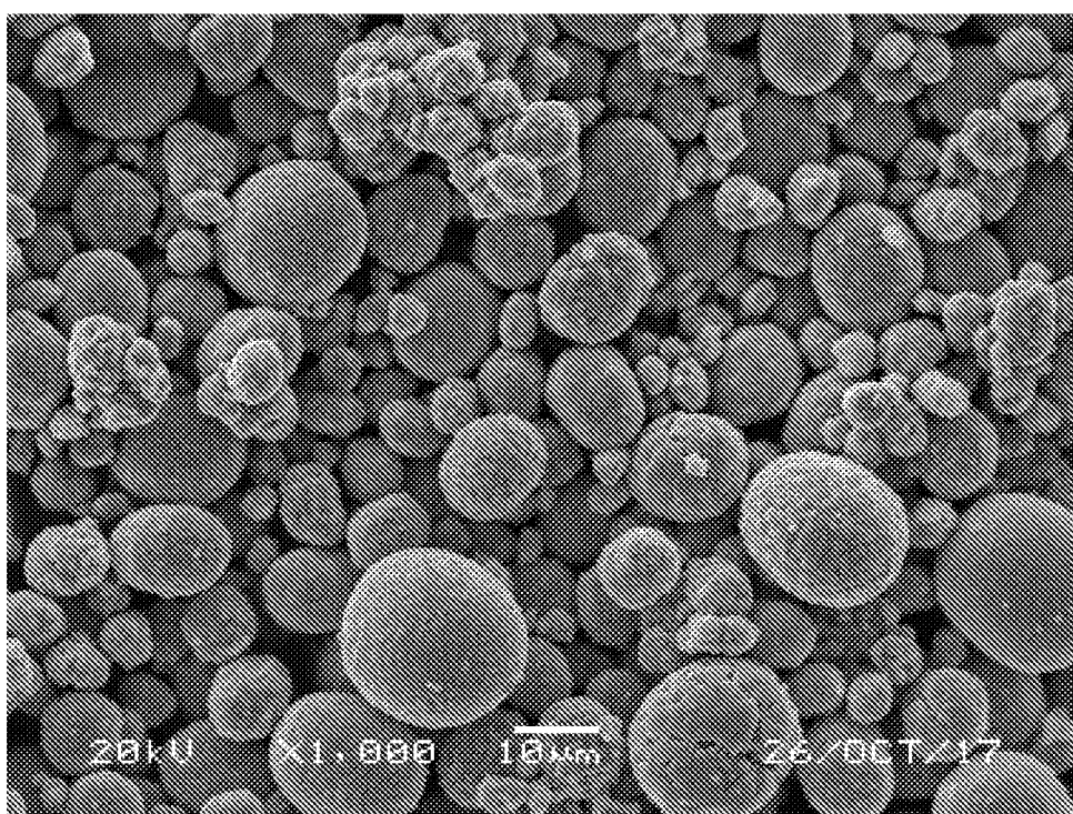
Fig. 7(d) Solid blending coating of \text{Li}_3\text{AlO}_{1.5}\text{F}_3 (Al:F:Al-O = 50:50 mol/mol) on NMC622 core particles
