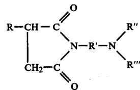
in which R is a hydrocarbon radical having a molecular weight ranging from about 280 to 1800, R' is a divalent hydrocarbon radical having from 2 to 10 carbon atoms and R" and R''' are hydrocarbon radicals having from 1 to 6 carbon atoms or are interconnected to form a heterocyclic ring consisting of from 3 to 6 atoms selected from the group consisting of carbon, nitrogen and oxygen atoms.
