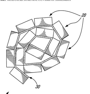
(57) Abstract: This invention relates to an improved surface covering assembly. The assembly consists of a plurality of elongated adjacent panels which, in a preferred embodiment, are attached to an elongated sheet of flexible material. The sheet can further comprise covering such as synthetic turf, carpet, etc. The surface covering assembly can thus be rolled/folded and unrolled/unfolded as desired. Multiple assemblies can be joined together to cover larger areas.
