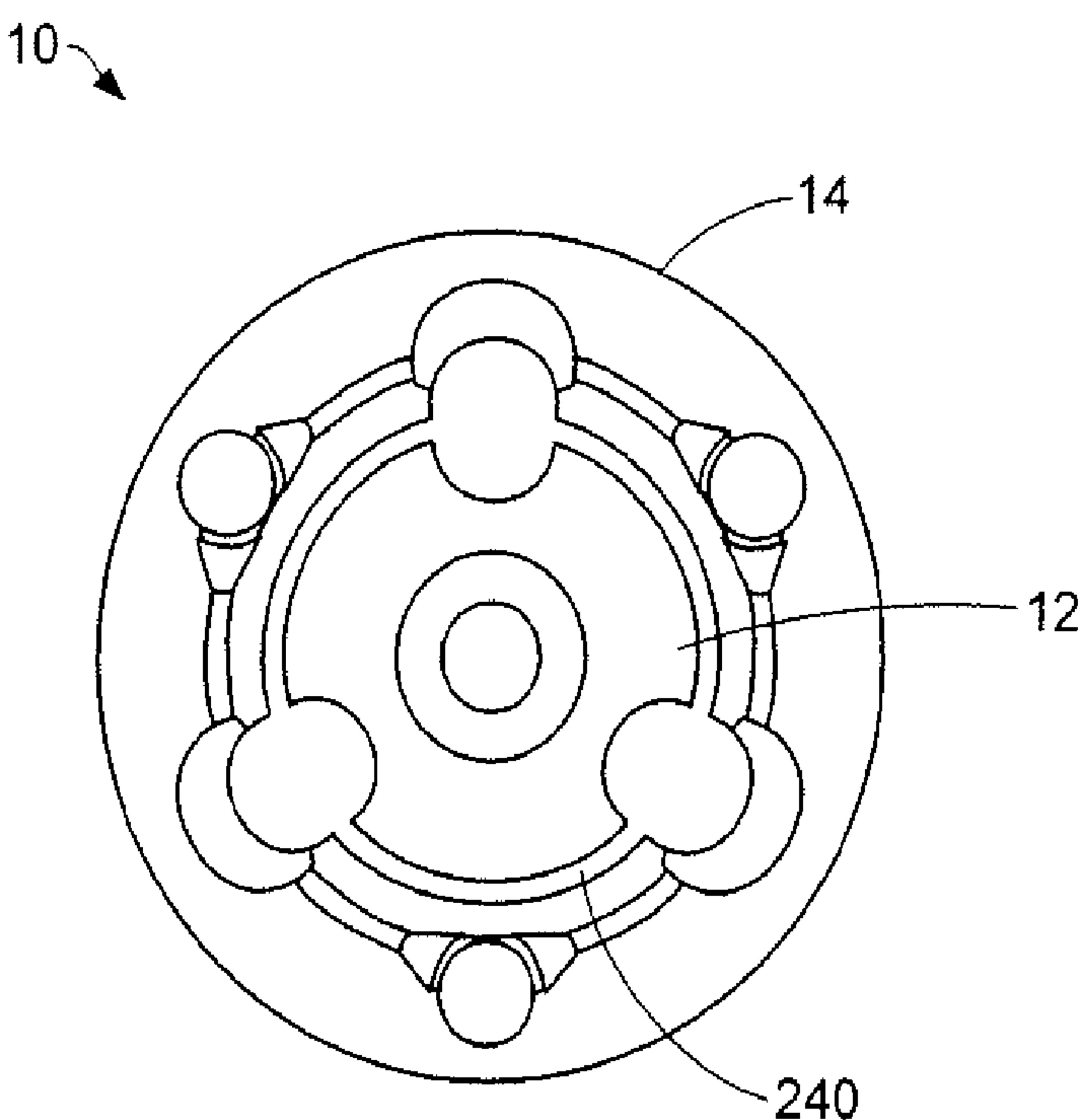
(57) Abstract: A steerable multi-linked device. The device includes a first multi-linked mechanism and a second multi-linked mechanism. The first mechanism defines a first plurality of grooves. The second mechanism defines a second plurality of grooves. The first and second pluralities of grooves cooperate to define at least two working ports along a length of the device. At least one of the first and second mechanisms are steerable.
