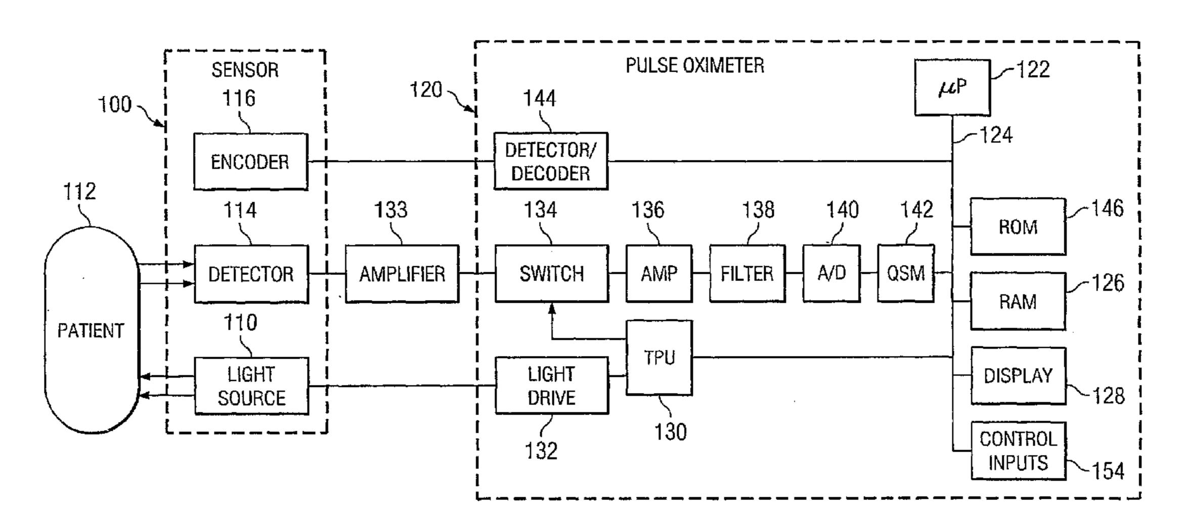
(57) Abstract: A method and a system for ensemble averaging signals in a pulse oximeter, including receiving first and second electromagnetic radiation signals from a blood perfused tissue portion corresponding to two different wavelengths of light, obtaining an assessment of the signal quality of the electromagnetic signals, selecting weights for an ensemble averager using the assessment of signal quality, and ensemble averaging the electromagnetic signals using the ensemble averager.
