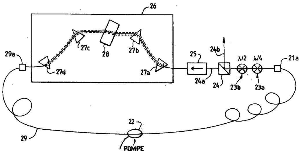
(57) Abstract: The invention concerns an ultrashort power laser pulse laser source, comprising an optical cavity (a) generating a pulse laser beam containing at least a gain medium (b), a non-reciprocal one-way operating element (d), and a system (e) compensating the cavity dispersion, and further comprises in the optical cavity a spectral-temporal spread mode locking device (c, 1, 26, 30).
