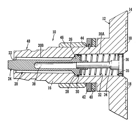
The present invention relates to a combined connector and valve which can be used in the evacuation of air from a closed space. In particular the invention is related to 5 manufacturing processes which are conducted in vacuum e.g. in the manufacture of fibre reinforced composites, in which a vacuum bag is used.
