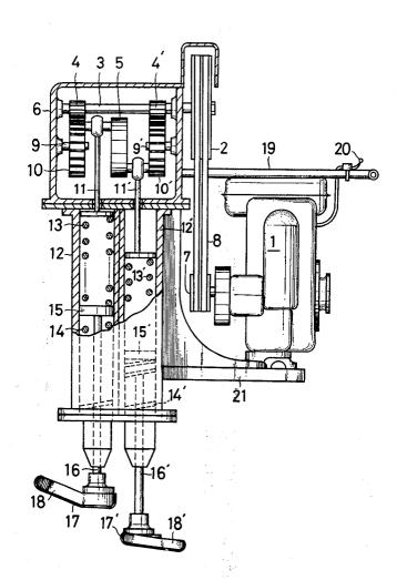
This invention relates to an earth tamper, and more particularly an earth tamper of two-vibration system which is capable of continuously tamping the earth for 5 compacting it.
