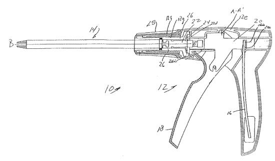
(57) Abstract: An instrument (10) for applying clips in surgery having an operating handle (12) with operating components and a clip cartridge with clip applying mechanism. The handle operating components generate reciprocal linear motion imparted to the clip applying mechanism and accommodate rotation of the cartridge about a cartridge axis. An anti-backup mechanism (24) constrains operating components to complete first and second strokes of reciprocal linear motion.
