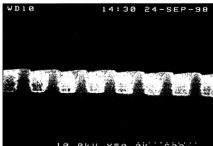
novolak underlayer with k=0.08 at 248nm
