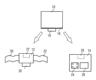
(57) Abstract: The invention relates to a modular microelectronic-system comprising: a first connection module (12) which can be firmly connected to user interface devices integrated into textile material; and a second connection module (14) which comprises user interface devices (24, 26) and/or which an be connected to an external device; in addition to an electronic module (10) which can be connected to the first connection module (12) or to the second connection module (14).
