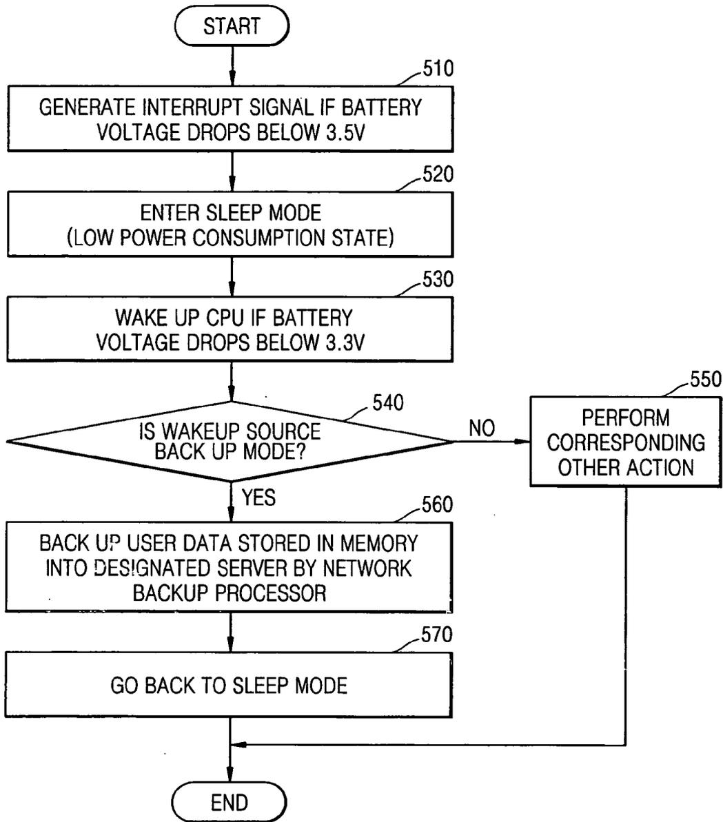
**METHOD AND APPARATUS FOR MANAGING POWER IN PORTABLE INFORMATION DEVICE**
