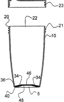
(57) Abstract: There is provided a spill proof cup assembly having a cap (24) with at least one spout outlet (26), a cup (10) with an upper open poriton (22) adapted to securely and sealing receive the cap (24), and a thermoplastic elastomer, or similar elastomeric material, co-molded bottom portion (40) with a vent disposed therein for allowing air to enter the cup as fluid exits through the spout outlet. The result is a one-way flow of air.
