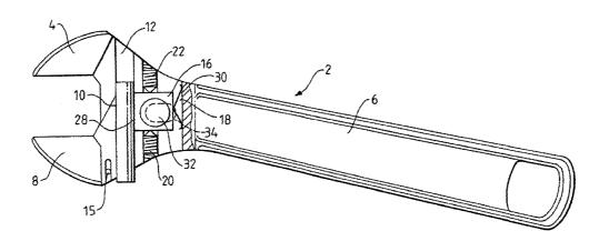
(57) Abstract: The present invention relates to an adjustable spanner (2) having a first fixed jaw (4) and a second moveable jaw (8). The second jaw (8) can be locked in fixed relation to the first jaw (4) by a locking means (16). This locking means (16) is moveable between a first position in which the second jaw (8) is fixed in relation to the first jaw (4) and a second position in which the second jaw (8) is permitted to move with respect to the first jaw (4).
