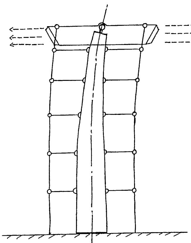
**(57) Abstract:** The invention concerns a radio broadcasting device consisting of a relay tower whereof the top part supports at least an antenna connected to an electronic equipment comprising a HF amplifier characterised in that said electric equipment is arranged in the top part of the relay tower.
