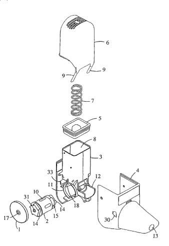
(57) Abstract: A multiple-dose powder inhaler is disclosed comprising an inhaler body defining a medicament container, an air channel, a mouthpiece, a rotatable metering drum with one or more peripheral dosing recesses and a dose counter for indicating the number of metered doses of medicament that have been dispensed from, or remain in, the medicament container. The inhaler is useful e.g. in the treatment of asthma.
