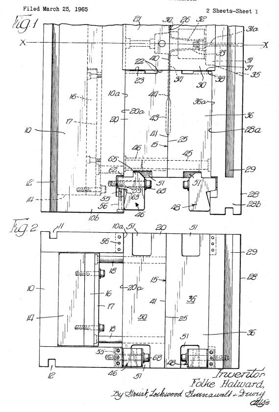
CLAMP FOR UNIT DIE MECHANISM
