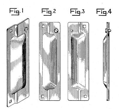
FIG. 1 is a front perspective view of a protective latch cover showing my new design.
