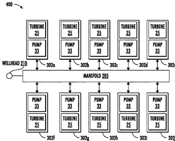
operating one or more units at MCP level and operating one or more units at Maximum Intermittent Power (MIP) level to meet the demand HHP signal.
